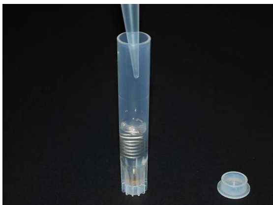
3: Fill the tube with 4.9 mL Extraction Solution
