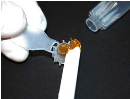
1: Fill the beaker with sample and wipe off excess sample
