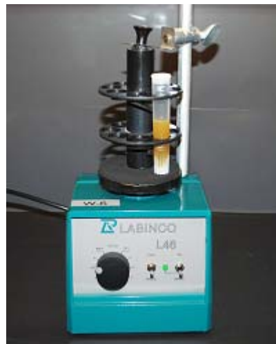
4: Vortex vigorously (1000 rpm) for three minutes.
